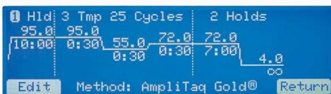
Time and temperature profiles show up clearly on the backlit display as you program them. While your method is running, you can track its progress in real time.
